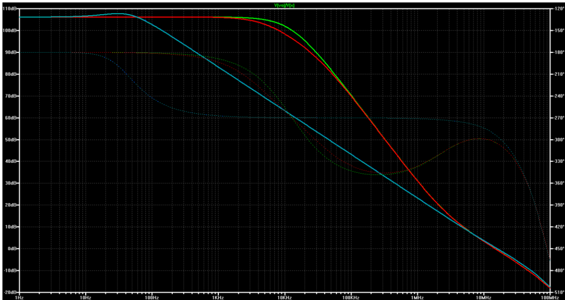
Figure 6 - Loop Gain Response ( A_{cl} = 16 \text{ dB} )
