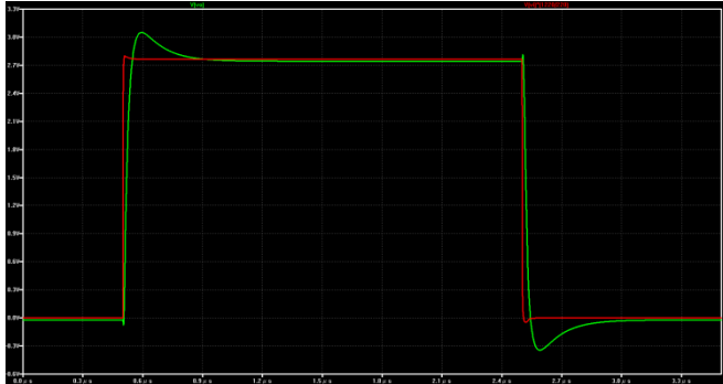
Figure 7 - Stepped Response (500mV input)
