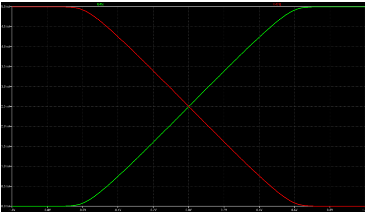
Figure 5 - Input Stage Linearity Range
