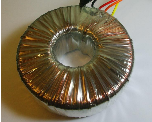
Photo 3 - e-Amp 1kVA Torroidal Transformer
